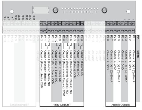
") Configuration of relay output terminals as per standard factory setting (NAMUR status signals)
